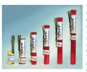
The NXbursT<sup>™</sup> 28 mm cartridges are used for boulder breaking; armour stone splitting; medium sized concrete demolition; dimension stone quarrying; swimming pools excavation and other sensitive in-situ breaking. The NXbursT<sup>™</sup> 28 mm Cartridge was designed specifically for underground applications where 32 mm holes are drilled horizontally. The NXbursT<sup>™</sup> 28 mm Cartridge is available in 20 grams to 120 grams charge-weights in increments of 20 grams.
