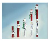
NXbursT<sup>™</sup> RockPoppers are used for breaking small boulders up to 1 cubic metre in size (used widely in breaking crusher oversize); scale removal in tanks and silos; and small demolition jobs. They require a 14 - 16 mm diameter hole which can be drilled with a hand-held electric hammer drill.
