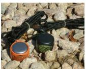
**BC-T 4 Haptic Bridge Wire Continuity Tester.** It has an astoundingly low (55 micro amps) maximum testing current and a robust feedback. The continuity is indicated via a strong tactile vibration ( that is felt through gloves).
