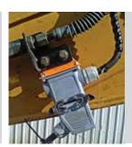
**Quick Connect** - Should it been needed, the MDA Drill is fully removable with two pins, two hydraulic quick disconnects, and one electrical quick disconnect.
