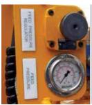
Adjustable Feed Pressure - The MacLean MDA Drill Feed features adjustable feed pressure. Just set the pressure for the rock conditions and begin drilling!
