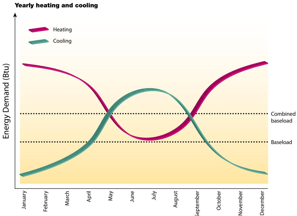
**Figure 10:** This graph is a typical annual combined heat and cooling load profile. This shows higher heat demand during the winter months and higher cooling demand during summer months when heat demand is low.
