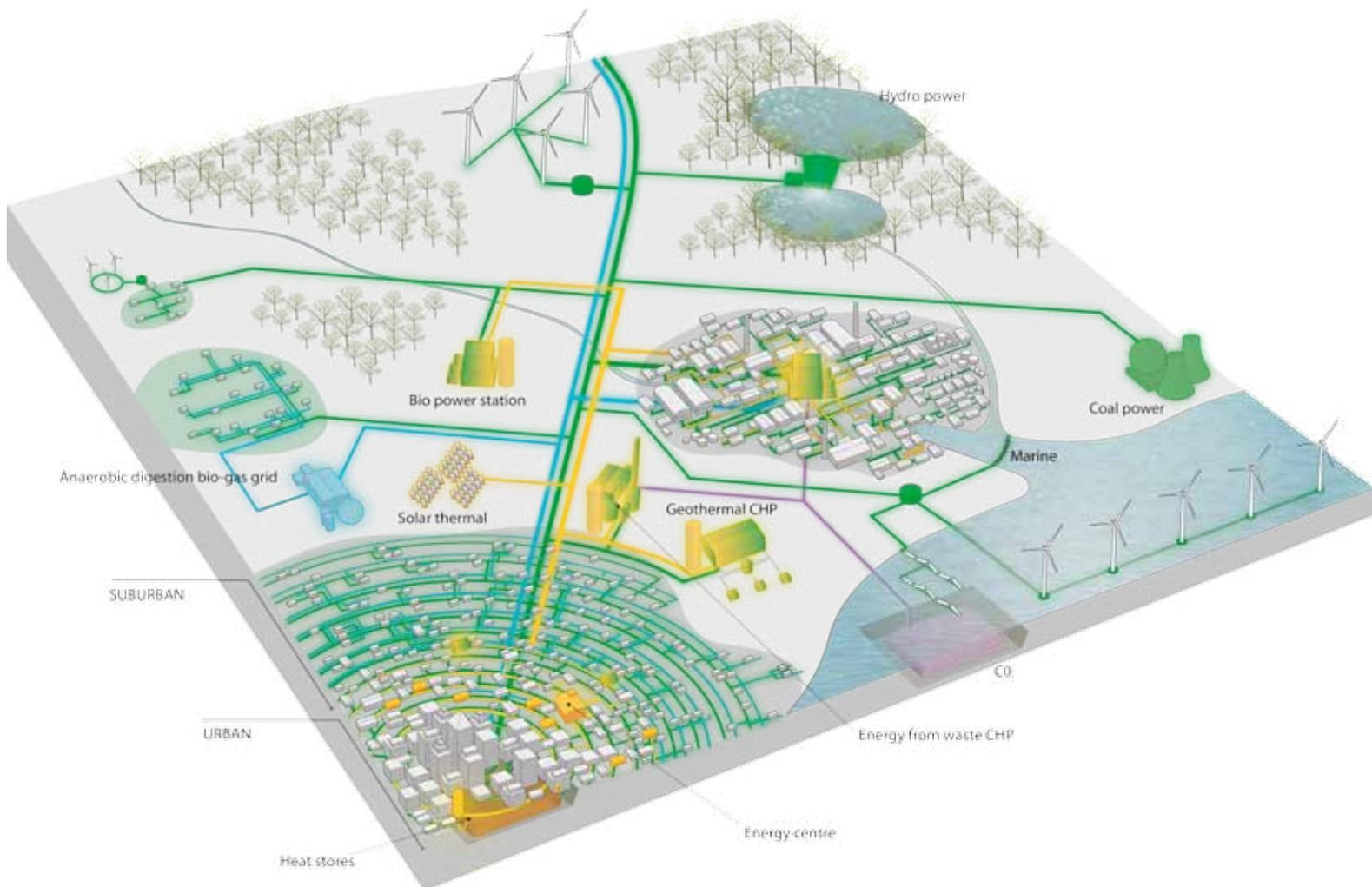
**Figure 14:** District energy infrastructure allows communities to capture thermal energy from a wide range of sources.
