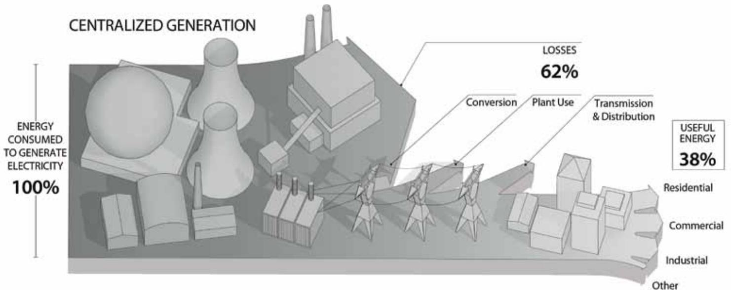
**Figure 2:** The typical centralized power generation process wastes approximately two-thirds of primary energy in the form of heat rejected into the atmosphere. District energy captures this heat and is 80–90% efficient.
