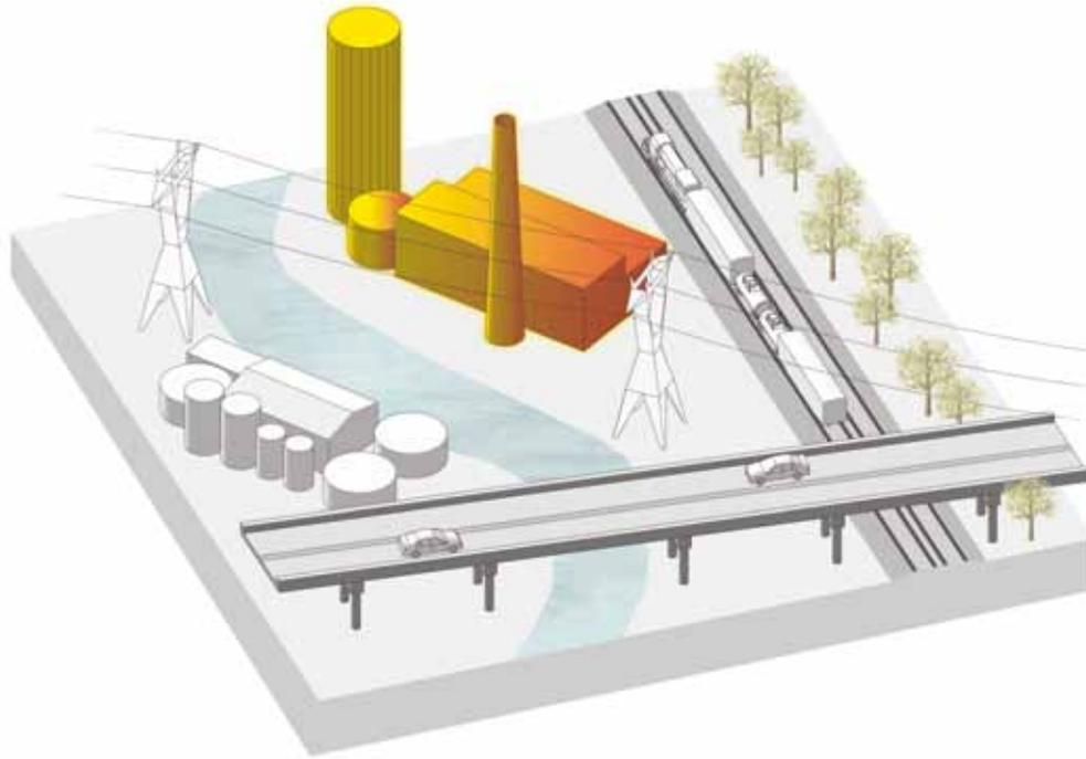
**Figure 11:** Potential barriers must be identified and taken into consideration. These might be: railway lines/subways, storm water drains, highways, canals, or rivers.
