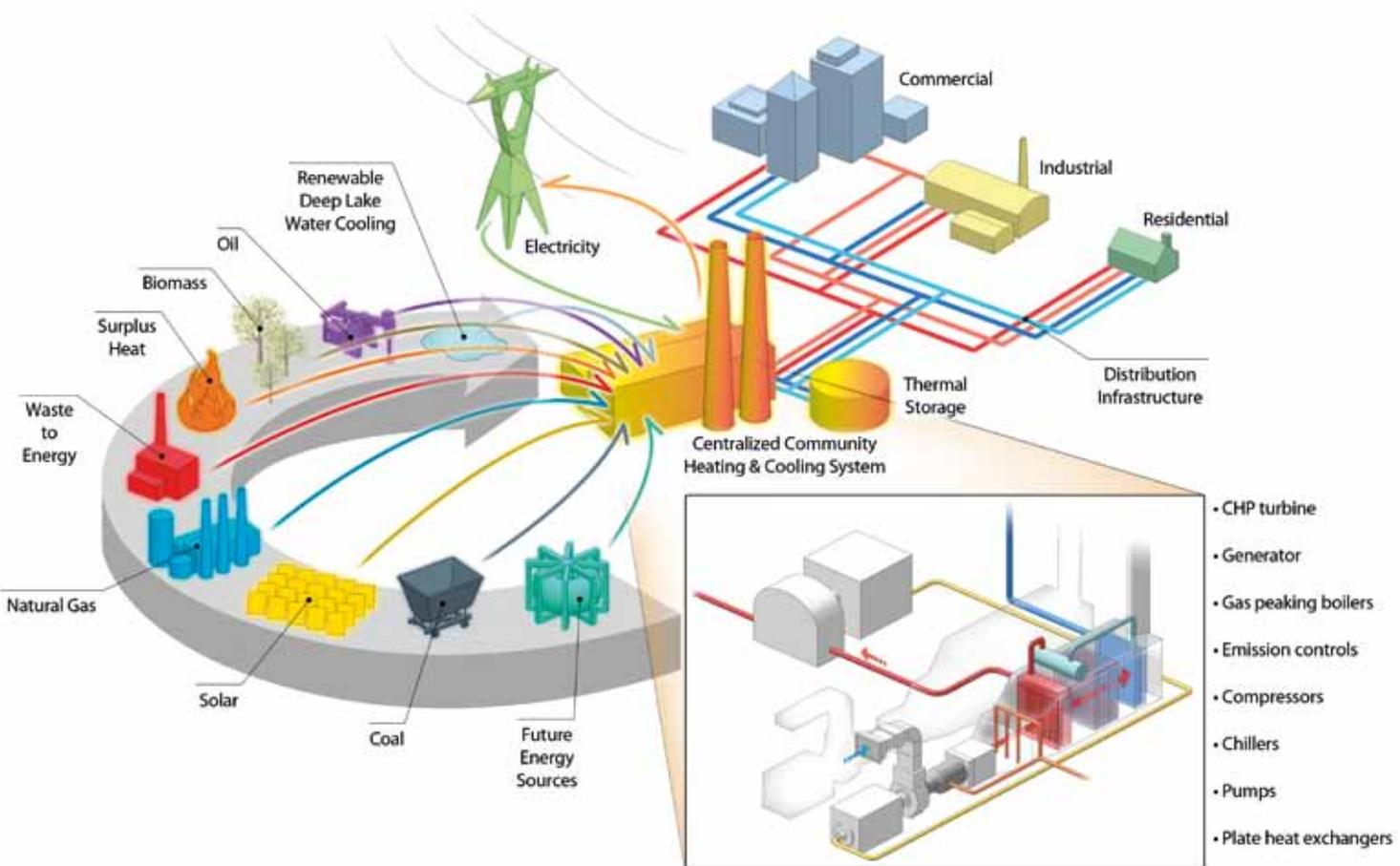
**Figure 16:** District energy can integrate a variety of fuel sources to take advantage of market conditions and local resources. The central plant houses the prime movers which will vary based on the plant design and configuration.
