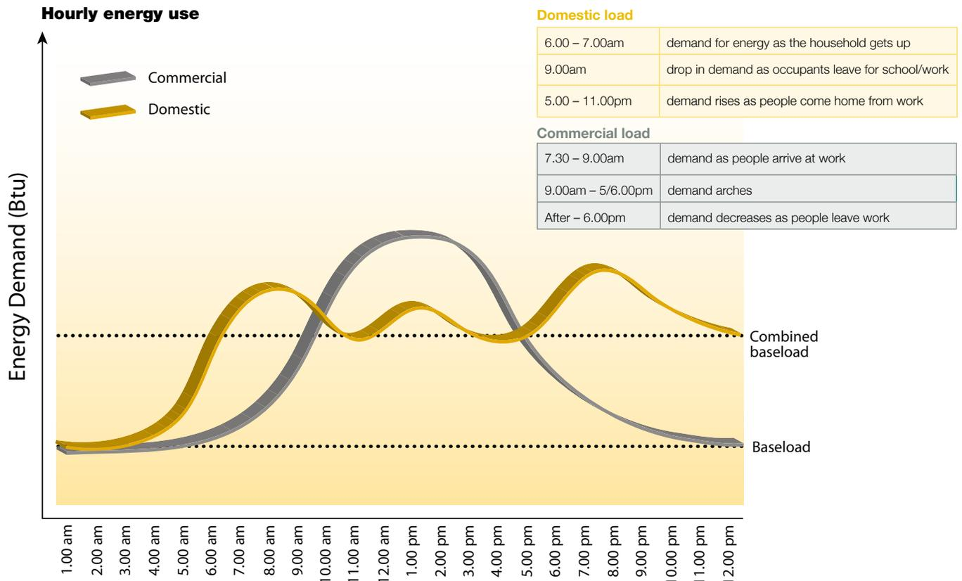
**Figure 9:** This graph shows a typical domestic and a typical commercial load profile, and how they complement each other.
