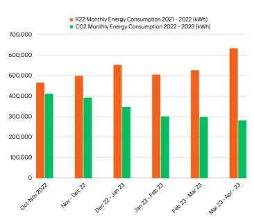
In order to ascertain the tangible energy savings resulting from the installation of CO<sub>2</sub>, a comprehensive analysis of energy bills spanning from October 2022 to April 2023 was conducted. These bills consistently revealed a notable **decrease in energy consumption of 129,627 kilowatt-hours (kWh)** in the six month period.
