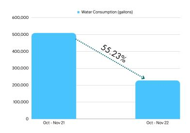
Moreover, in order to assess the effect of replacing the evaporative condenser with a new gas cooler on water consumption, a comparative analysis was conducted against the corresponding period in the previous year. It is worth noting that the cooling load remained constant throughout this evaluation. The results revealed a substantial **reduction** in water usage of approximately 55.23%, with consumption decreasing from 509,520 gallons in the previous year to 228,130 gallons.
