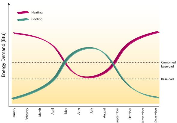
**Figure 10:** This graph is a typical annual combined heat and cooling load profile. This shows higher heat demand during the winter months and higher cooling demand during summer months when heat demand is low.
