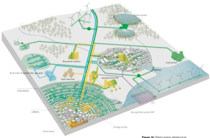
Figure 14: District energy infrastructure allows communities to capture thermal energy from a wide range of sources.
