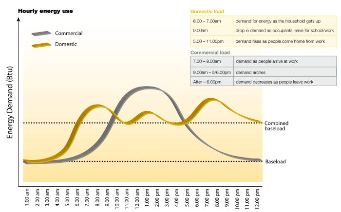
Figure 9: This graph shows a typical domestic and a typical commercial load profile, and how they complement each other.
