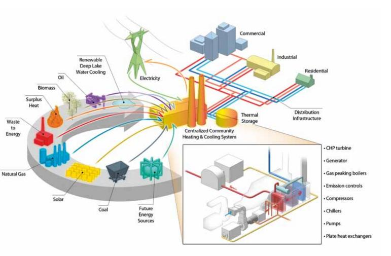
Figure 16: District energy can integrate a variety of fuel sources to take advantage of market conditions and local resources. The central plant houses the prime movers which will vary based on the plant design and configuration.
