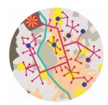
**3.** Networks begin to link to each other to share excess heat capacity. Original heat sources are replaced as they reach the end of their life, potentially with waste heat from a power station. A transition main will carry large volumes of heat over long distances.
