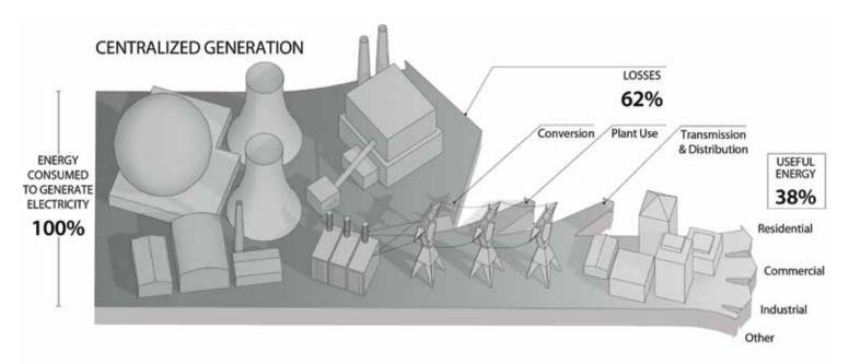
**Figure 2:** The typical centralized power generation process wastes approximately two-thirds of primary energy in the form of heat rejected into the atmosphere. District energy captures this heat and is 80–90% efficient.
