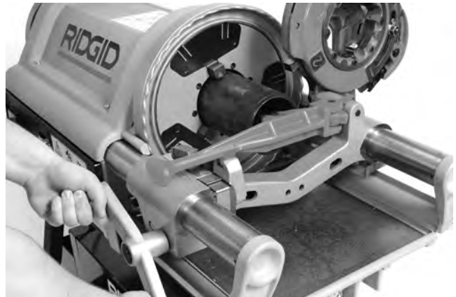
Figure 22 – Reaming Pipe with Reamer
