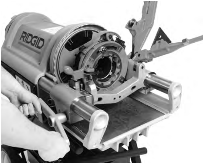
Figure 23 – Threading Pipe (714 Die Head Shown)
