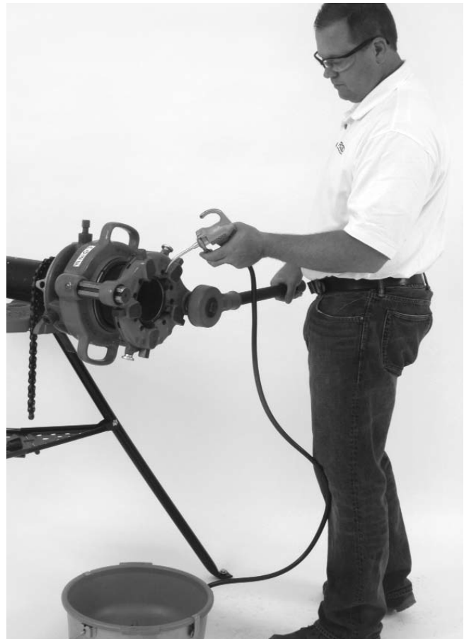
Figure 7 – D-1440 Ratchet Operation
