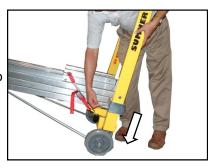
Fold the leg until it forms a 90 degree angle with the base
