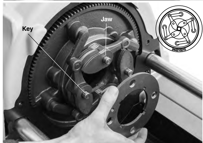
Figure 32 – Changing Auto Chuck Machine Jaws
