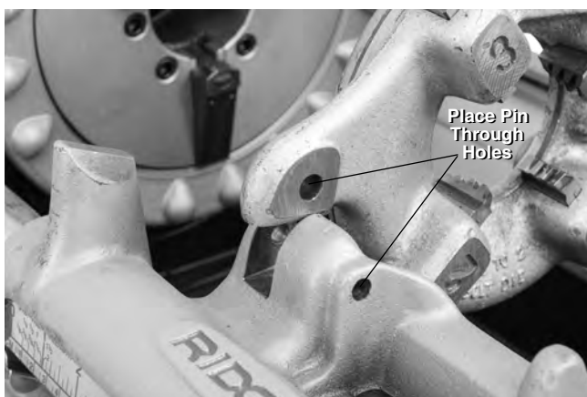
Figure 26 – Retaining LH Die Head in Place
