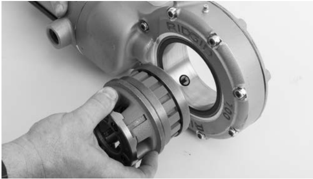
Figure 4 – Installing Die Heads into 700 Power Drive
