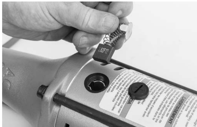
Figure 13 – Installation des balais
