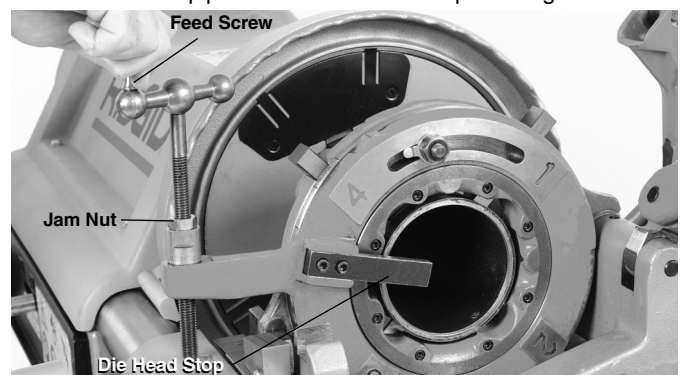
Figure 3 – Grooving the Pipe
