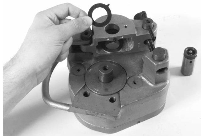
Figure 10 – Placement of Thrust Washer
