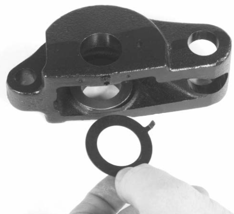
Figure 18 – Inserting Tabbed Thrust Washer
