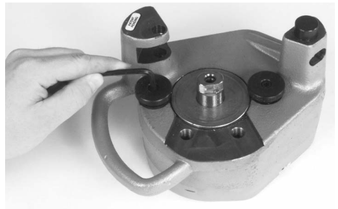
Figure 17 – Installing Copper Stabilizer Pad
