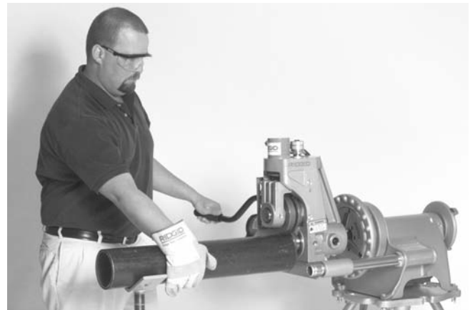
Figure 16 – Applying Pressure on Pipe with Power Drive in REV Mode.
