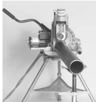
Figure 12 – Offset Pipe on 918 in FORWARD Position
