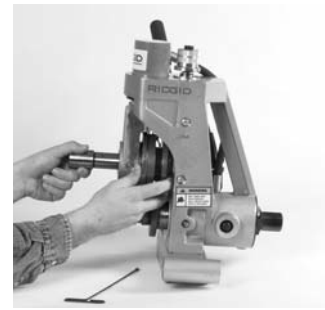
Figure 18 – Removing Retaining Shaft and Groove Roll
