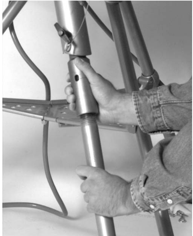
Figure 6 – Adjusting Legs to Level Groover
