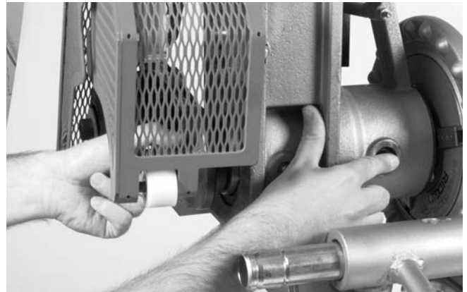
Figure 20 – Engaging Lock Pin and Removing Drive Roll
