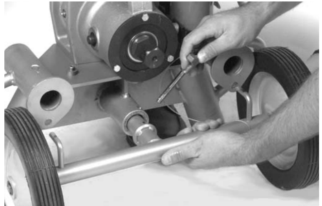
Figure 3 – Removing Transport Cart
