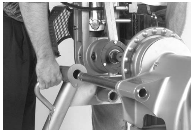
Figure 4 – Sliding Roll Groover Onto Support Arms
