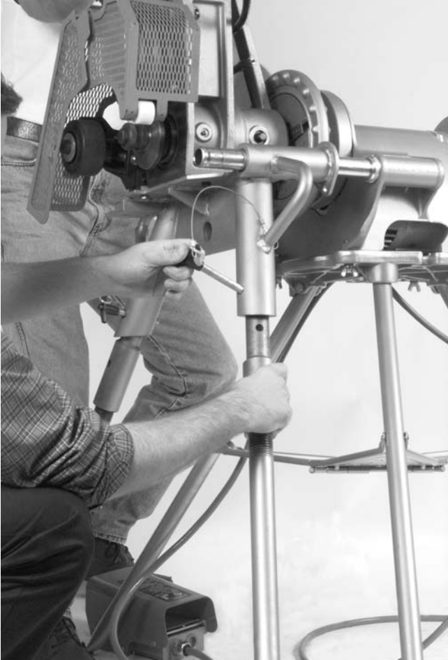
Figure 5 – Installing Legs Into the Groover Base
