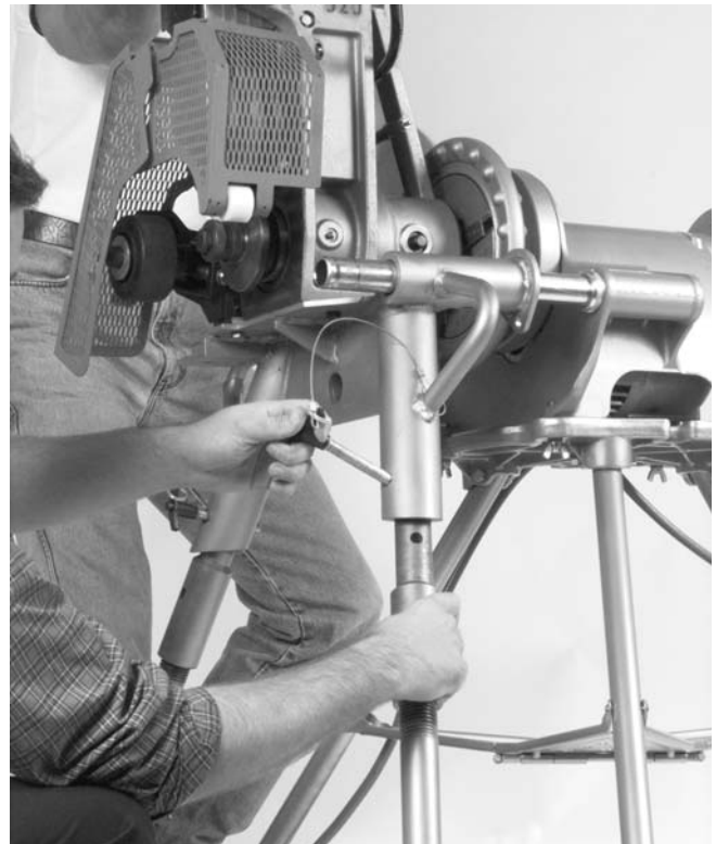
Figure 23 – Removing Legs From Base
