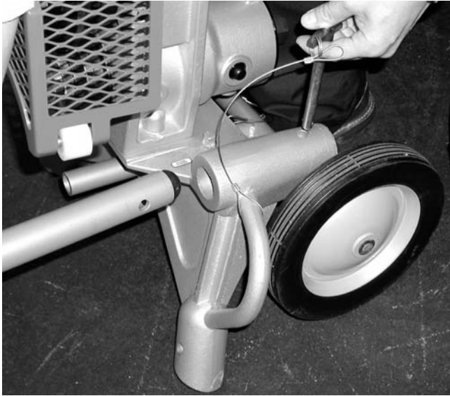
Figure 25 – Attaching the Support Legs
