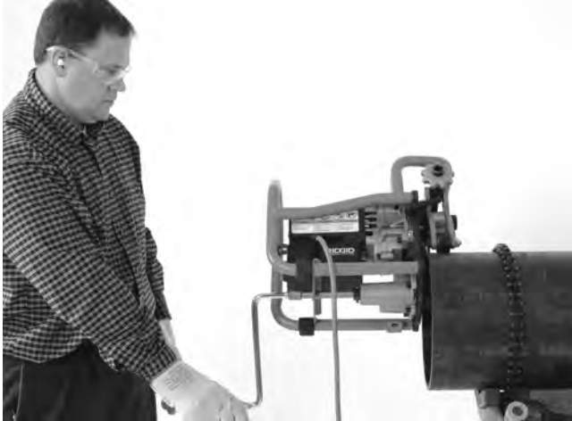
Figure 20A – Bevelling Operation (Fixed Workpiece/Moving Beveller)
