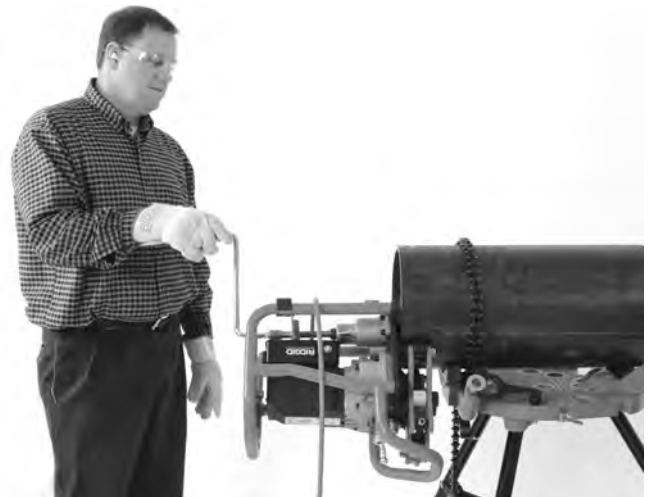
Figure 20B – Bevelling Operation (Fixed Workpiece/Moving Beveller)
