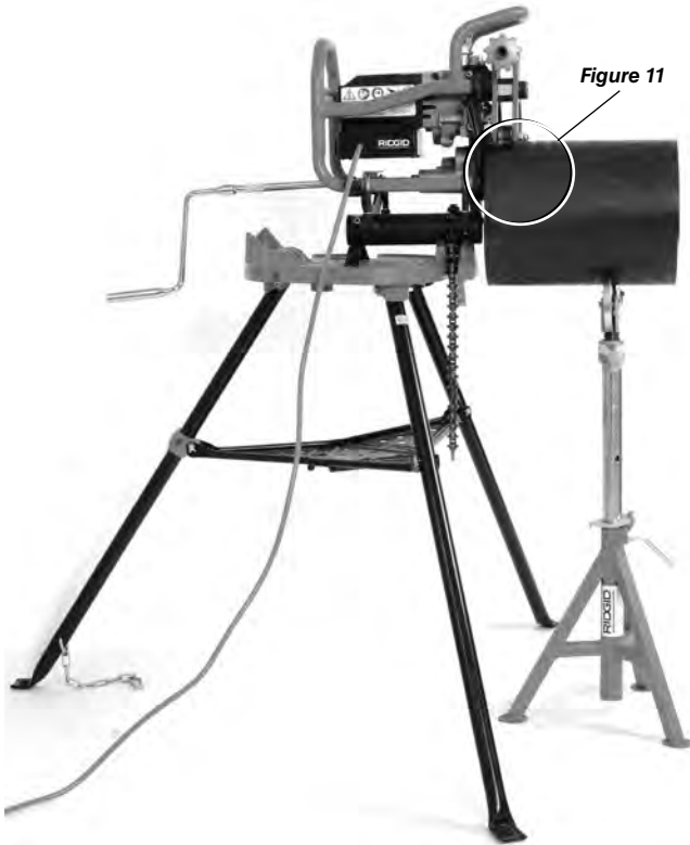
Figure 12 – Machine fixe, tuyau court, un porte-tubes
