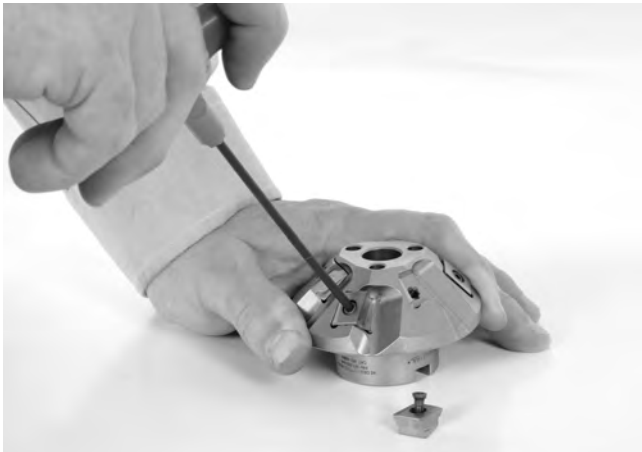
Figure 24 – Replacing Cutter Inserts
