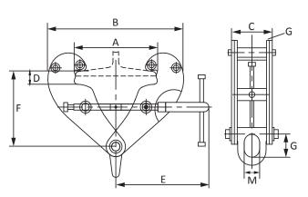
This I-beam clamp can be used as an anchor for various applications and for any type of construction. The 'eye' shackle design assists the user in rigging, and the zinc plated clamp screw assembly allows for easy adjustment of the clamp. This clamp features metric capacities that range from 1, 2, 3, 5, and 10 tons.
