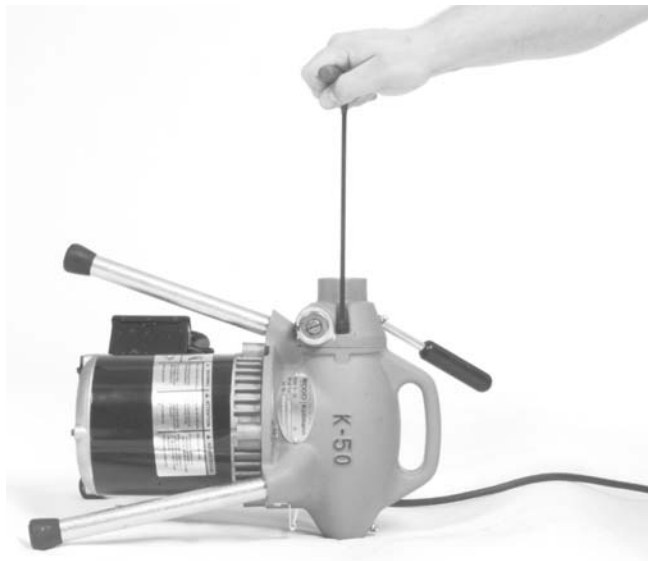
Figure 10 – Remove Socket Head Cap Screws
