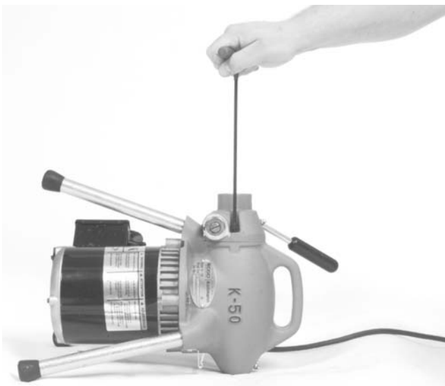
Figure 10 – Retrait des vis Allen
