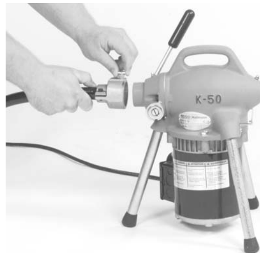
Figure 2 – Rear Guide Hose Attachment
