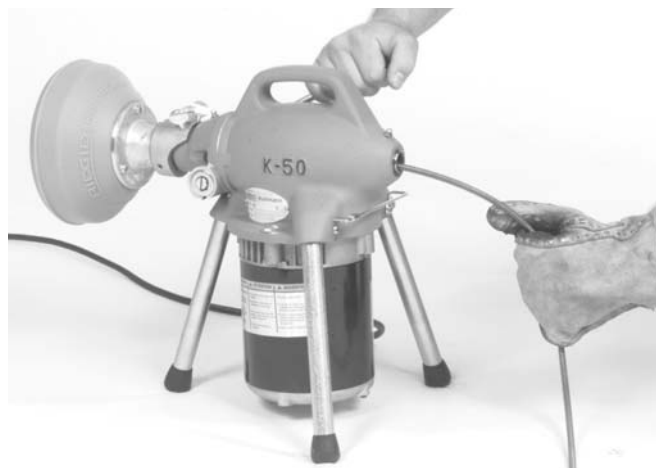
Figure 5 – Cable Adapter Attachment
