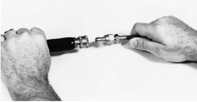
Figure 3 – Connect jetter hose to jetter
