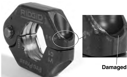
Figure 11 – Damaged Ring Pocket
