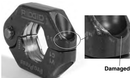
Figure 11 – Damaged Ring Pocket
