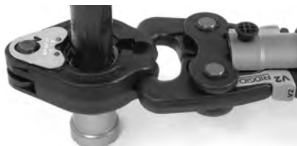
Figure 12A – Placing Actuator Tips Into MegaPress Ring Pockets
