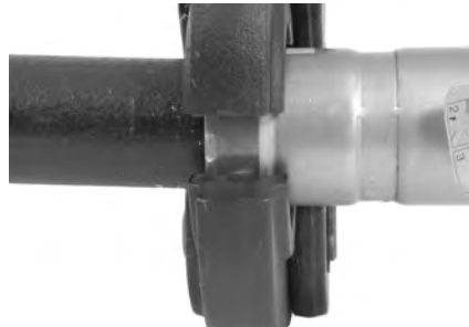
Figure 9 – MegaPress Jaw Set Square To Fitting and Tubing
