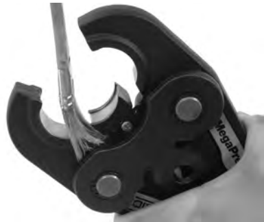
Figure 13 – Cleaning Segment Area of MegaPress Jaw
