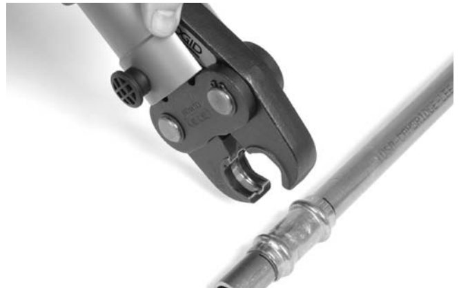
Figure 6 – Opening The Scissor-Style Jaw Set
