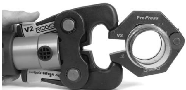
Figure 9 – Attaching Actuator to Press Ring
