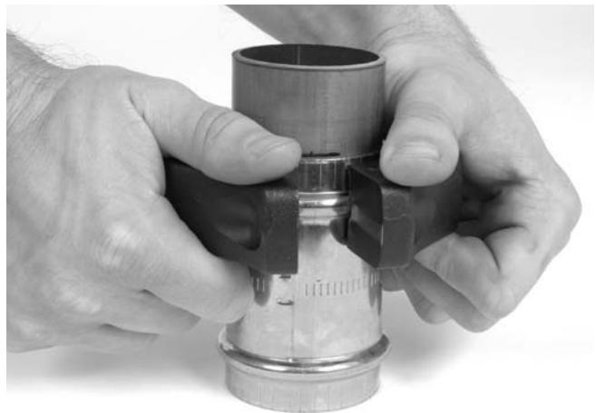
Figure 8 – Installing Press Ring Onto Fitting
