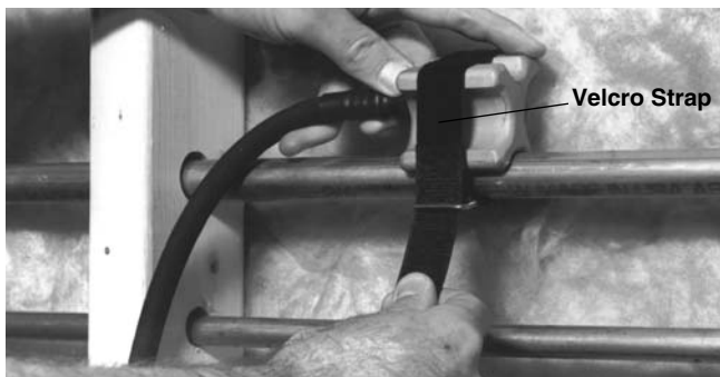
Figure 5 – Applying Freeze Head with Velcro Strap
