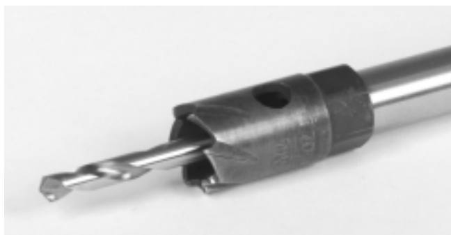
Figure 5 – Installation of pilot drill
