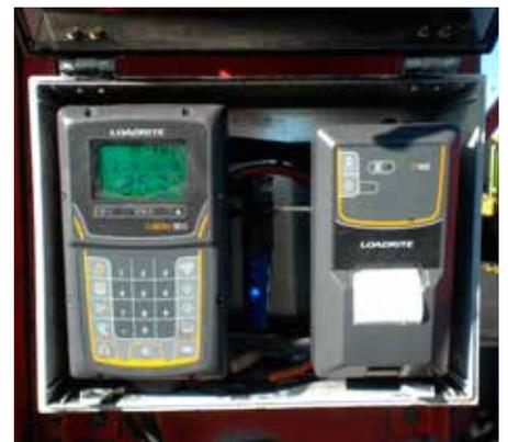
C1850 and printer protected within an enclosure
