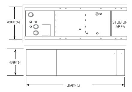
Tanks are UL Listed and constructed in accordance with UL Standard for Safety UL 142, Steel Aboveground Tanks for Flammable and Combustible Liquids and Canada CAN/ULC Fabricated Steel above ground Horizontal Tanks for Flammable and Combustible Liquids.
