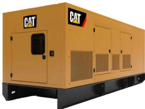
These sound attenuated, factory installed enclosures incorporate internally mounted super critical level silencers, designed for safety and aesthetic value on integral fuel tank base or optional dual wall integral fuel tank base for total fluid containment. These enclosures are of extremely rugged construction to withstand exposure to the elements and provide weather protection.
