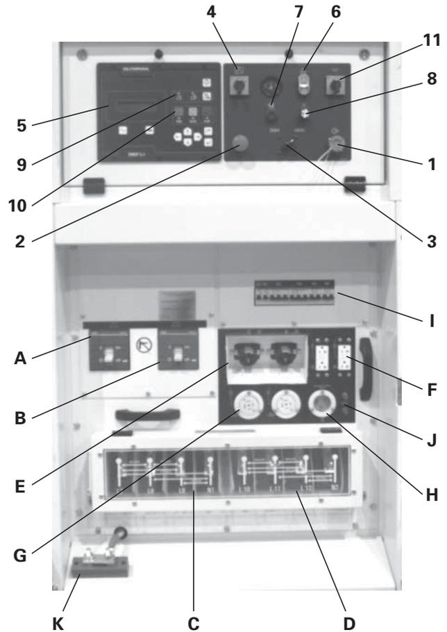
\* Either set of bus bars is capable of supplying up to full rating. Total load from bus bars and receptacles cannot exceed rating of generator set. Generator is wye connected in all cases.
