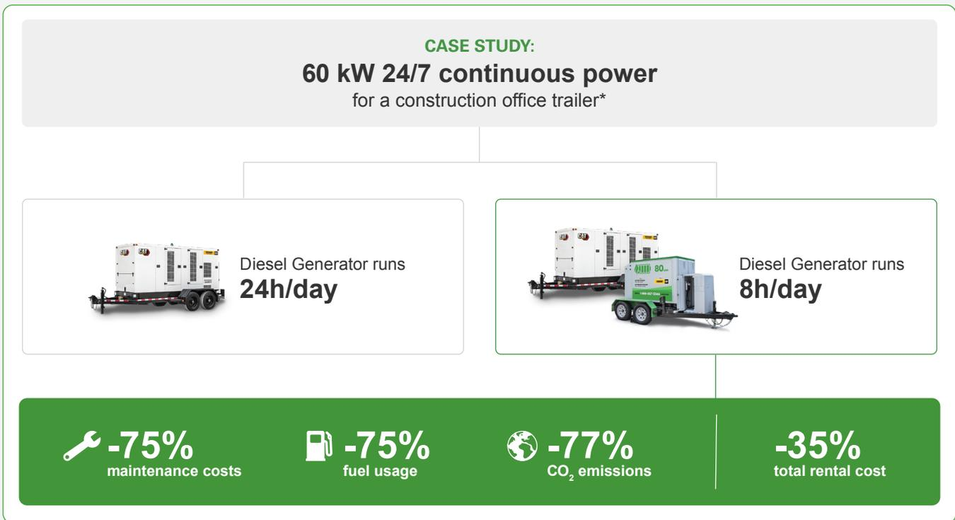
\*Estimated results based on Toromont Cat case study for a typical 60kW 24/7 continuous power requirement, comparing a triple-shift diesel generator versus a single-shift diesel generator plus BESS unit.
