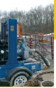
Gorman-Rupp sets the industry standard in heavy duty solids-handling trash pumps for all your construction and rental needs. These pumps feature a removable cover plate that provides easy access to the impeller for inspection or service. Every pump is factory-tested for long lasting, troublefree operation.
