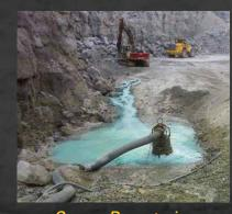
Quarry Dewatering 8" S Series submersible pump
