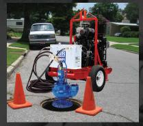
Hydraulic Submersible fits standard 24" manhole and passes a 5" solid
