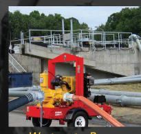
galvanized steel Bauer pipe with prime-assisted pump
